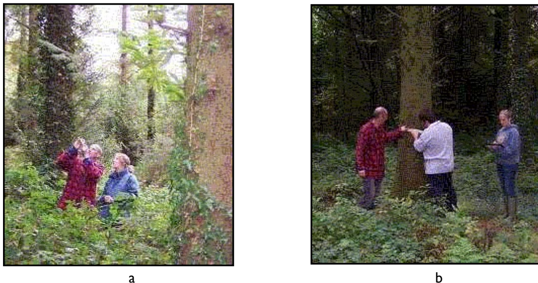
Fig. 1: A member of staff showing students how to use the clinometer (a) & the dbh tape (b).
